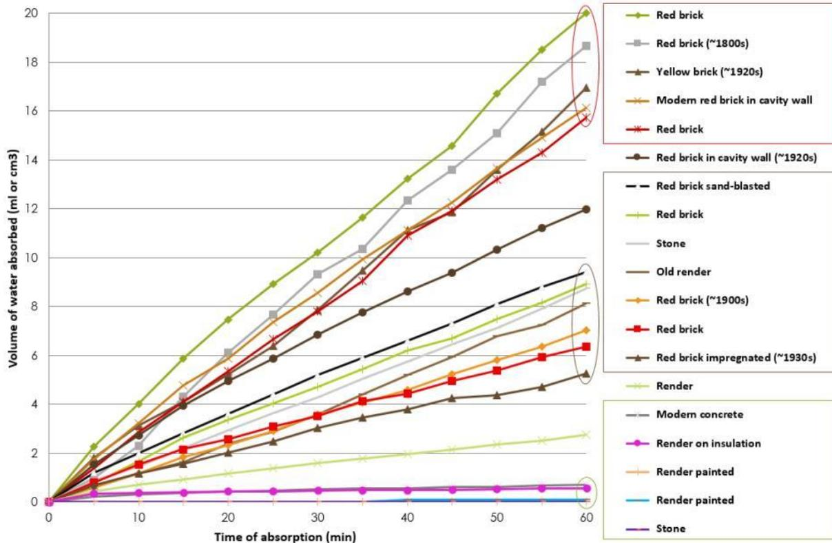
Figure 103 Absorption of a range of different buildings tested in Dublin: the mean progression is shown for each wall
