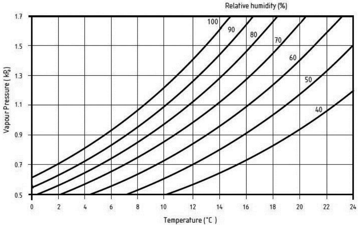
Figure 19 Simplified psychrometric chart showing the relationship between temperature (x-axis), vapour pressure (y-axis) and relative humidity (heavy lines): condensation will occur at 100 % RH, the graph of which indicates saturation vapour pressure and dewpoint temperature. (compare to Figure 18) (BSI, 2011, p. 21, fig. C.1/ Image © The British Standards Institution)
