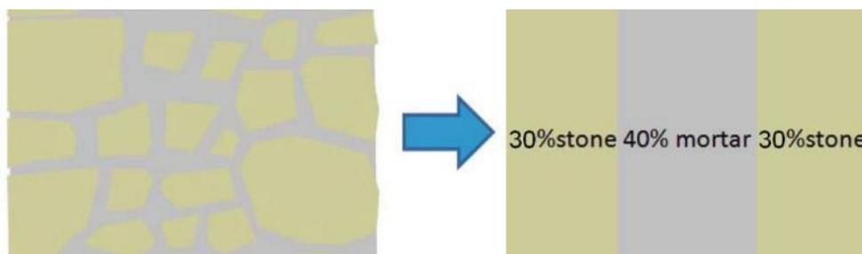
Figure 70 Simplified representation of a solid stone wall construction with a mortar core between two stone layers, as used for the hygrothermal assessments in this case study.
