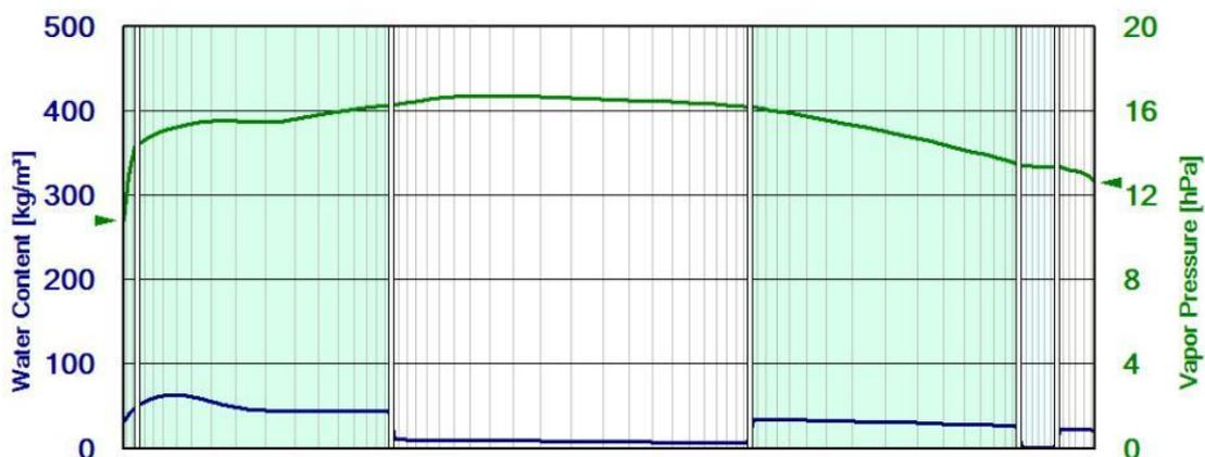
Figure 32 Diagram showing vapour pressure profile (green) and water content profile (blue) across a wall.
