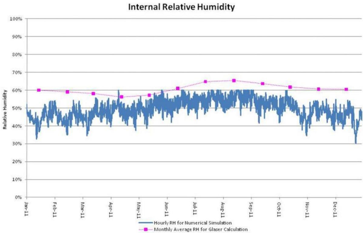
Figure 68 Indoor relative humidity data used for Glaser method and numerical simulations assessments
