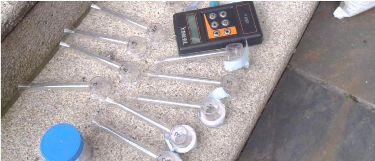
Figure 100 Karsten tubes, putty and Tramex MRH III moisture meter laid out ready for use.
