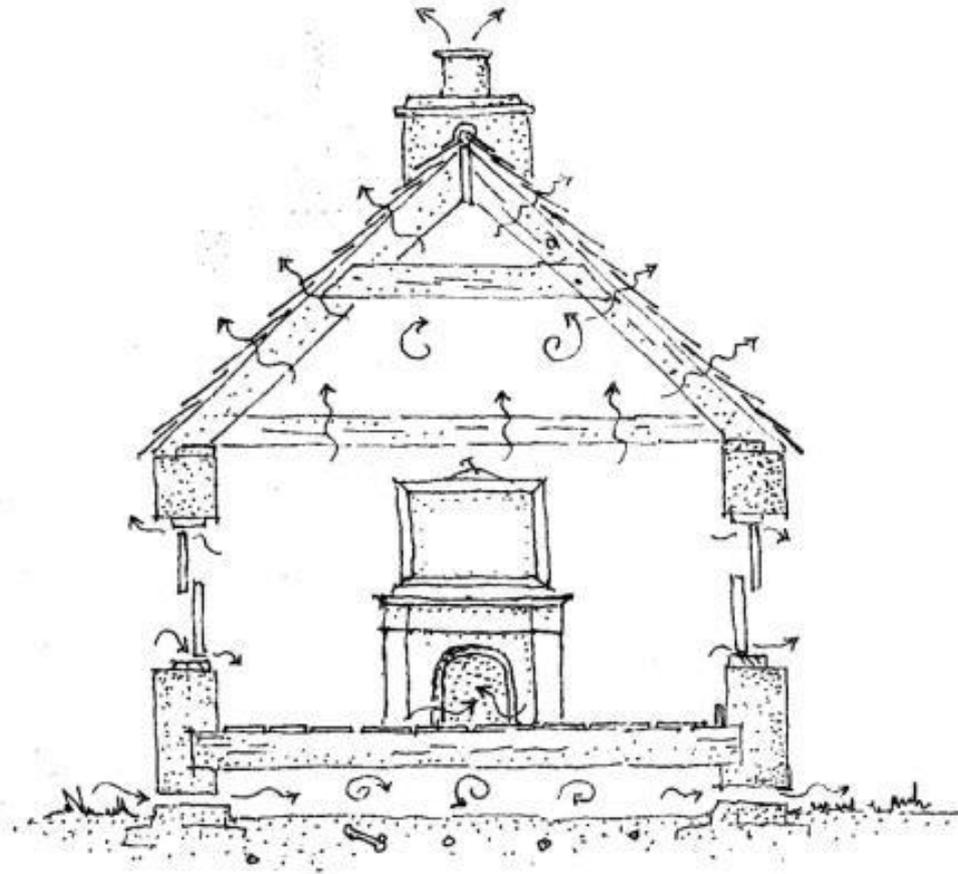
Figure 2 Sketch section illustrating how air moves into, out of and within a building.
