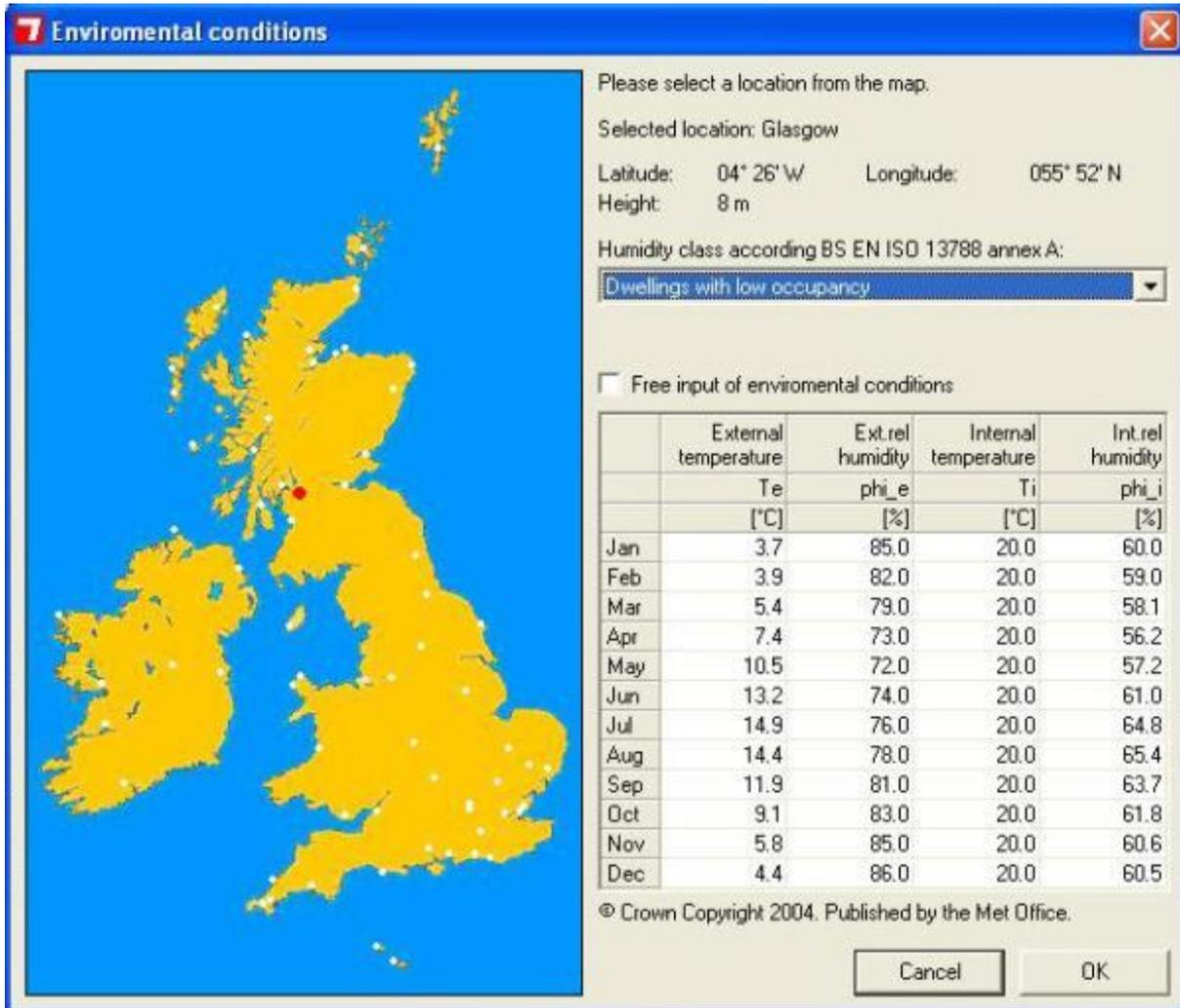
Figure 57 BuildDesk U screenshot showing the meteorological stations available for the British Isles and the environmental conditions available in the software for the location *Glasgow* with a humidity class setting of *Dwelling with low occupancy*.
