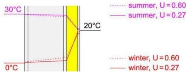
Figure 31 Steady-state temperature profiles for an internally insulated solid wall, with the internal wall insulation shown as yellow layer.
