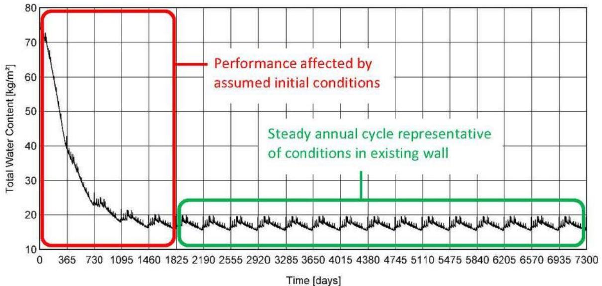
Figure 76 Total water content of base wall simulation with WUFI, for a 20 year simulation period (7300 days in total, with 365 days per year) to eliminate the influence of assumed initial moisture in the existing construction.
