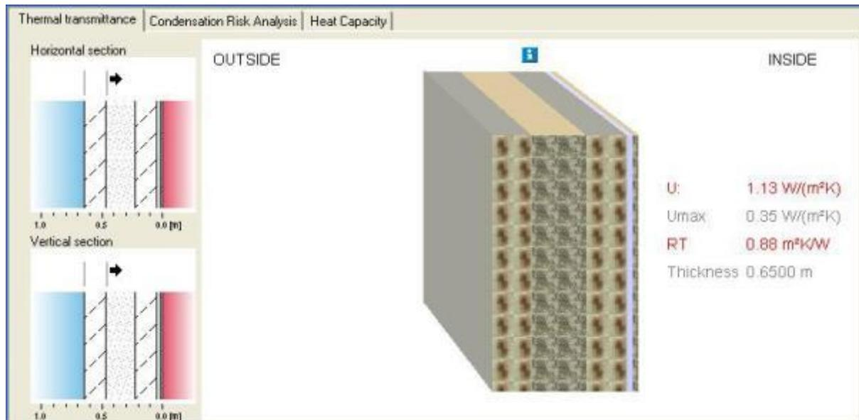
Figure 72 BuildDesk U screenshot showing model of the base wall with the following layers (starting on the left): stone, mortar core, stone, air space (light blue colour) and plaster
