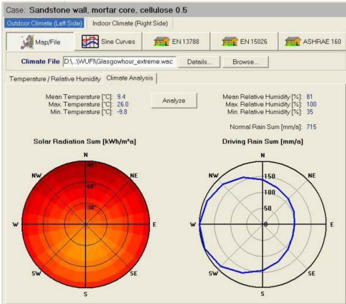
Figure 59 WUFI Pro screenshot showing basic climatic analysis of solar radiation and wind-driven rain for the location Glasgow
