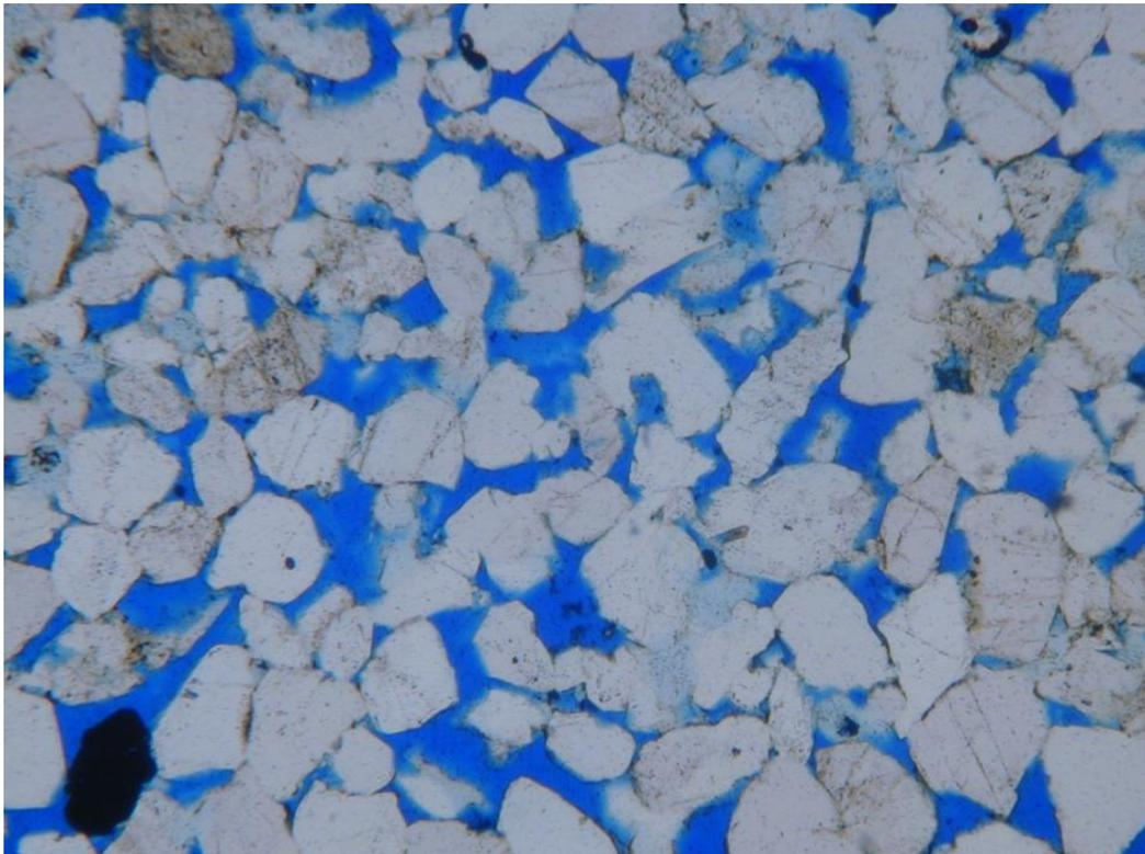
Figure 5 Scanning electron microscope photograph of a sandstone sample, cut, polished and coloured in blue to highlight its pore structure: the photo is of 10 x magnification, with the horizontal view approximately 3 mm wide
