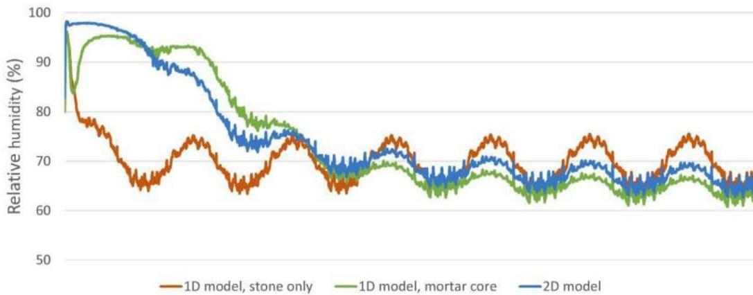
Figure 84 Relative humidity of the three wall models, at the interior wall surface (plaster surface), generated with WUFI for a seven year simulation period
