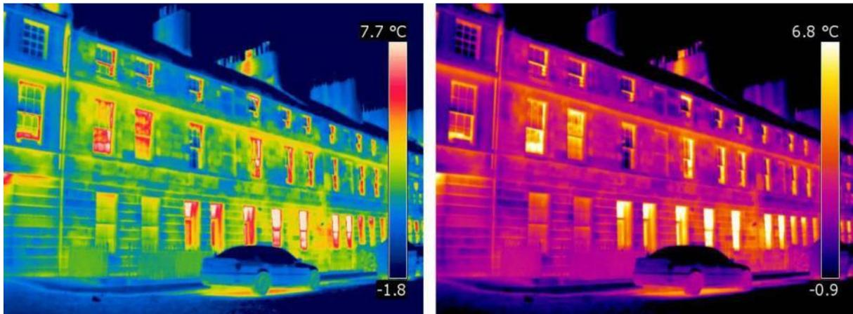
Figure 12 Two versions of a thermogram (infrared image) with different colour schemes and temperature ranges applied
