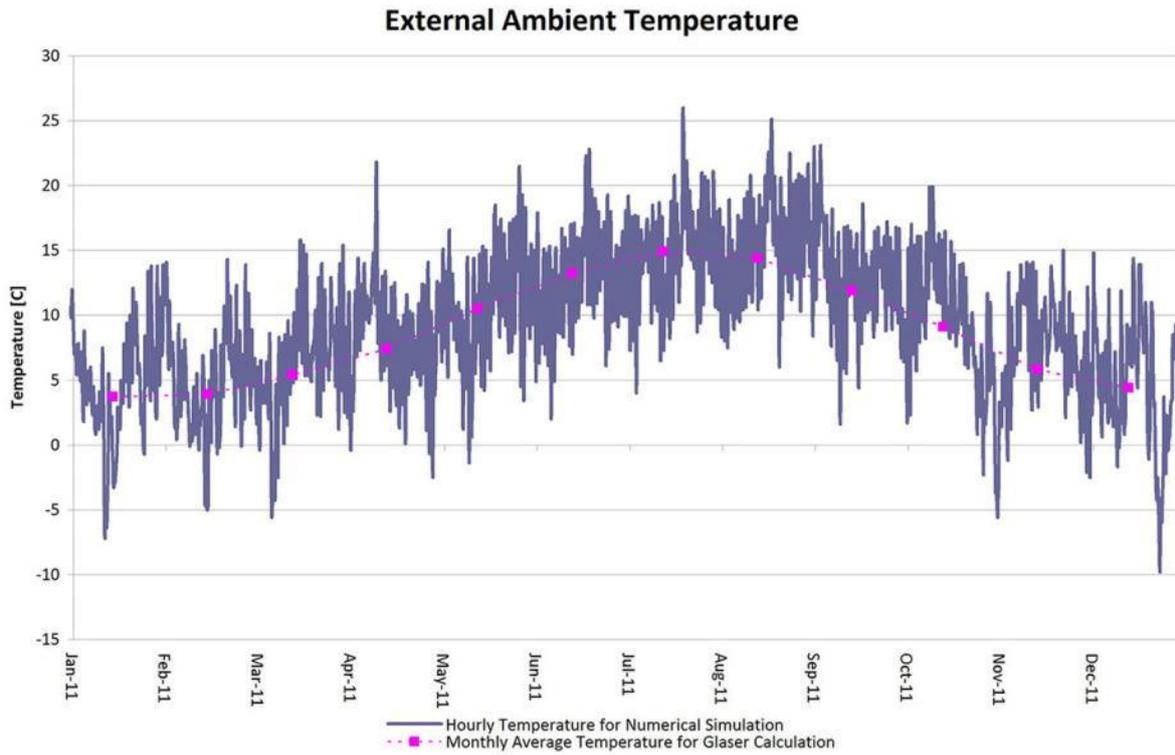
Figure 62 External temperature data used for Glaser method and numerical simulations assessments
