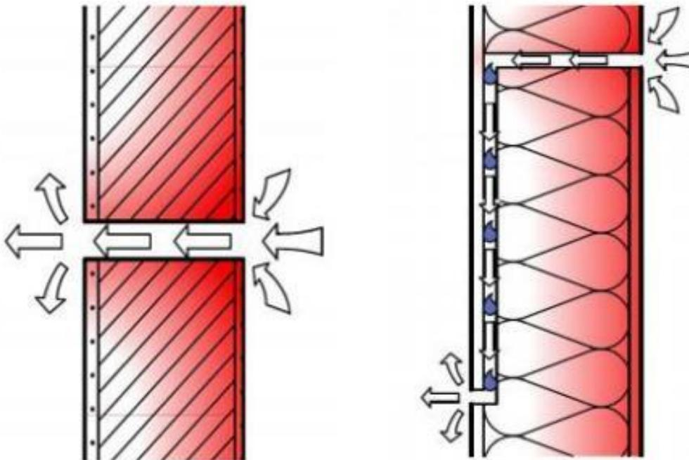
Figure 36 Air leakage through gaps and cracks in the building envelope: whereas through large gaps (left), air escapes rapidly, in small gaps with tortuous air paths, vapour can condense, as it is transported more slowly through the colder parts of the building fabric. (Künzel, 2011 / Image © Fraunhofer-Gesellschaft)
