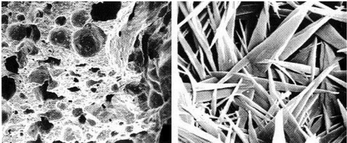
Figure 7 Scanning electron microscope photograph of aerated concrete with 22 x magnification (left) and 11,000 x magnification (right). (Krus, 1996 / Image © Fraunhofer-Gesellschaft)
