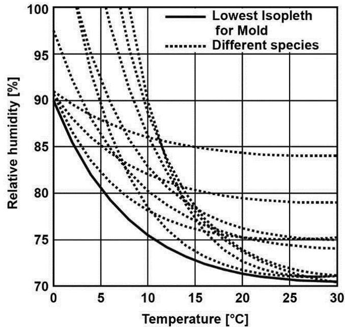
Figure 42 Example of isopleth models: the dotted curves describe the mould growth thresholds for different mould species. The overall threshold is the LIM graph, shown as continuous curve. (Sedlbauer, 2001, fig. 30 / Image © Fraunhofer-Gesellschaft)
