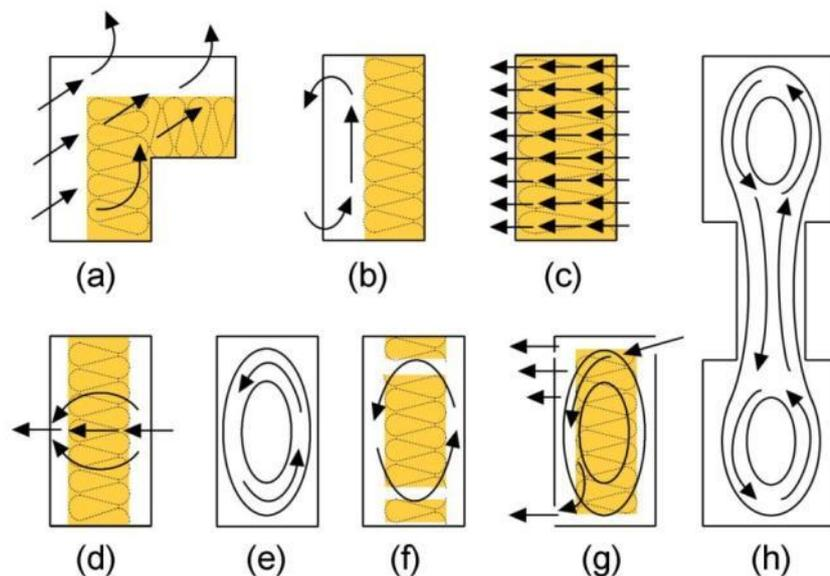
Figure 34 Examples of thermal bypass through or within building envelopes (indoors is on graphic's right side): The internal air barrier is compromised only in cases c, d and g. In the other cases, even with proper air barriers and good airtightness, air movement occurs within the building fabric, causing convective heat loss. (Siddall, 2009 / Image © AECB)
