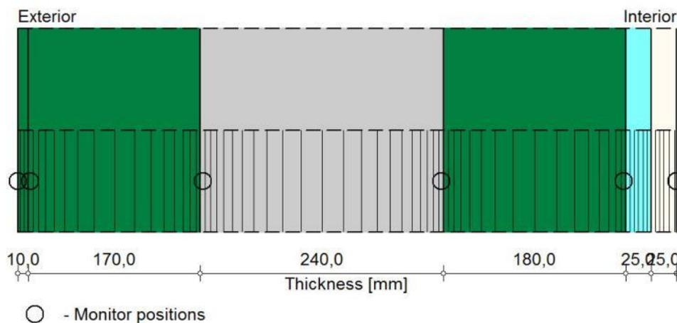
Figure 75 WUFI screenshot (excerpt) showing model of the base wall with the following layers (starting on the left): stone, mortar core, stone, air space (light blue colour) and plaster.
