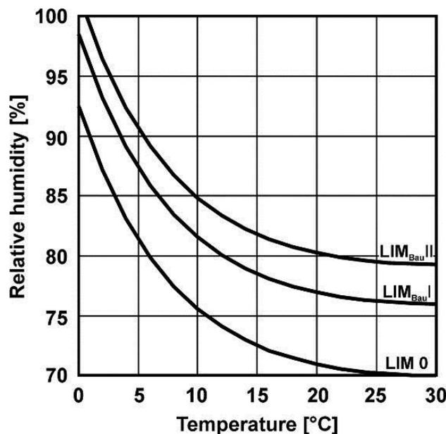
Figure 43 Example of LIM isopleths for different substrate classes for building materials: Curves LIM<sub>BauI</sub> and LIM<sub>BauII</sub> represents substrate classes I and II respectively; curve LIM 0 represents an ideal growing-substrate. (Fraunhofer IBP / Image © Fraunhofer-Gesellschaft)
