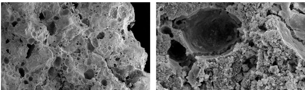
Figure 8 Scanning electron microscope photograph of mortar with 50 x magnification (left) and 2000 x magnification (right)
