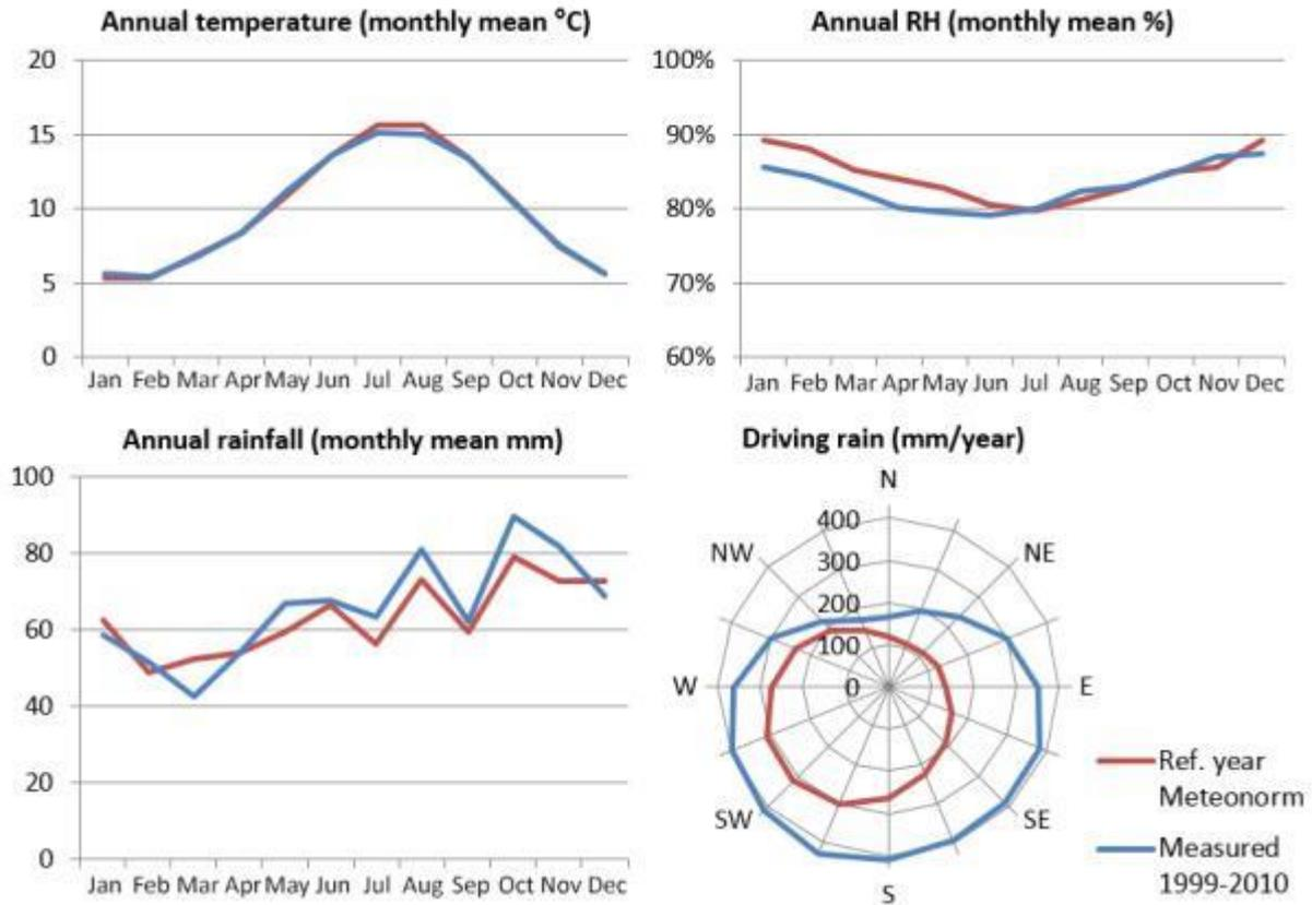
Figure 61 Comparison of synthetic climate data from a reference year in Meteonorm (red) and the related measured data from 1999 to 2010 (blue), both for Dublin Airport. Temperature, relative humidity and rainfall are averaged by month, while wind-driven rain is averaged by year over different directions.
