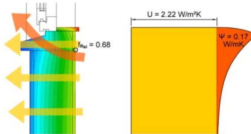
Figure 50 Diagrams illustrating heat flow at a thermal bridge: the junction between a wall and a window, with a cill in between. The left diagram, generated with THERM 5.2, shows the temperature variation across the fabric's cross section, overlaid with arrows for linear and non-linear heat flow (orange and yellow respectively). The right diagram shows the associated heat flow, with linear heat flow in yellow and non-linear heat flow in orange.
