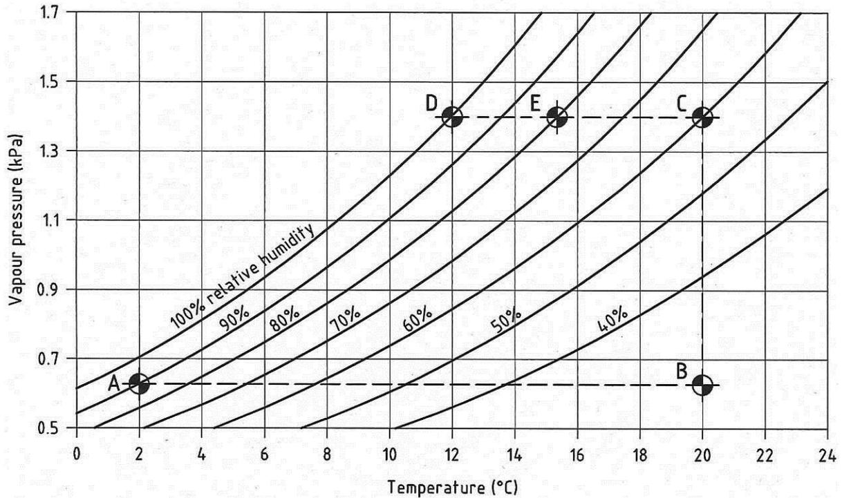
Figure 20 Psychrometric chart with five points (A to E) illustrating exemplarily how to read such charts. (BSI, 2011, p. 21, fig. C.1/ Image © The British Standards Institution)
