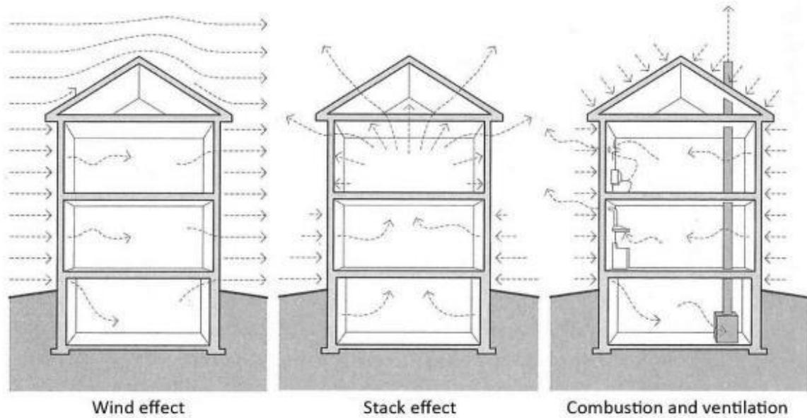
Figure 3 Natural and man-made forces driving air flow through building envelopes. (Straube and Burnett, 2005, p272, fig. 7.2 / Image © Building Science Press)
