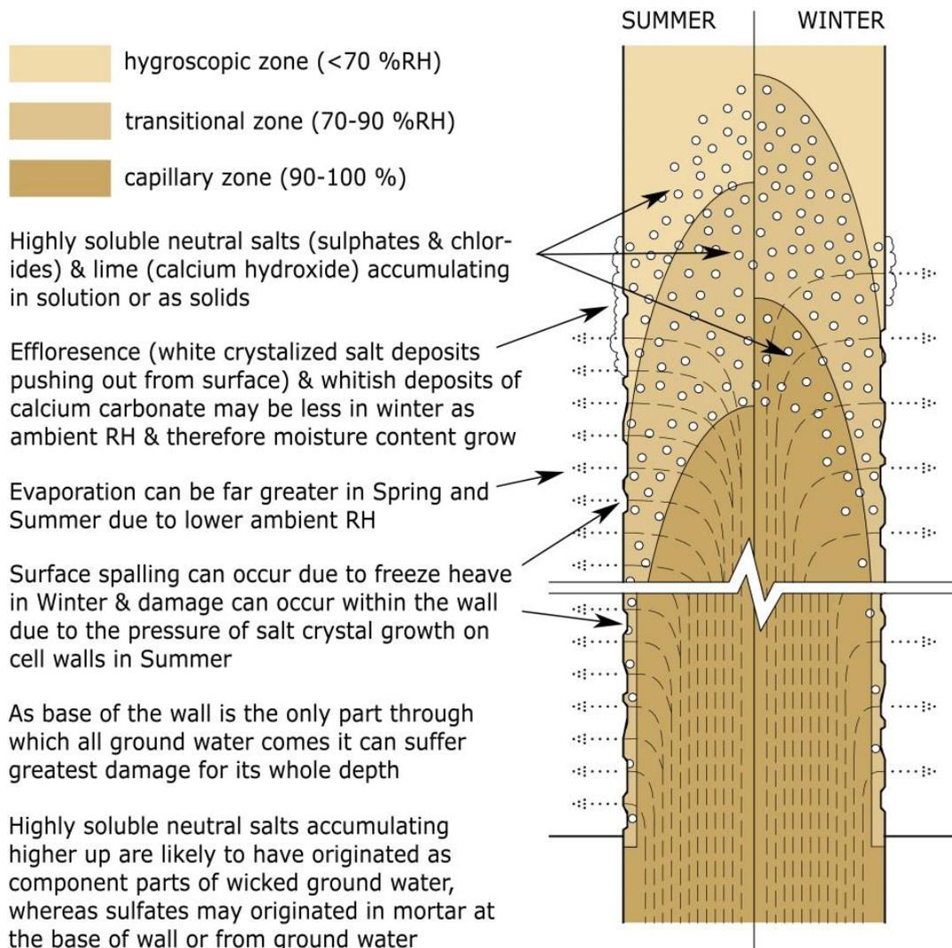
Figure 40 Diagram showing a wall cross-section with cyclical seasonal nature of rising damp and associated salt migration
