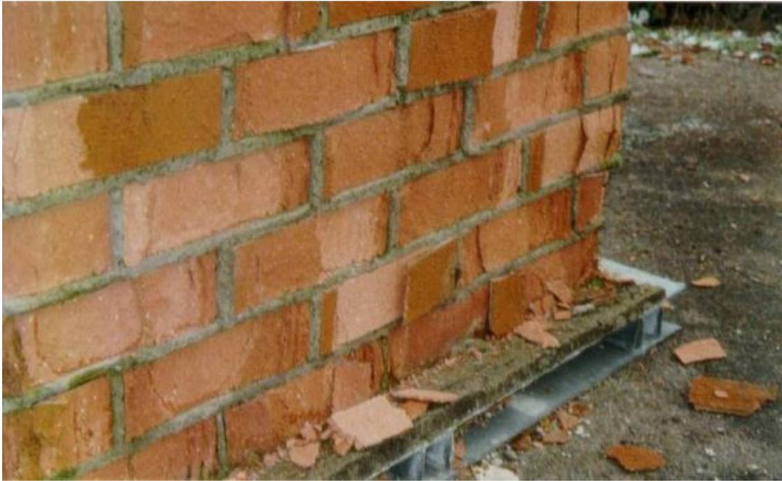
Figure 44 Surface spalling at a wall made from engineering bricks: It was wetted repeatedly under controlled climatic conditions to simulating freeze-thaw action. (Fraunhofer IBP / image © Fraunhofer-Gesellschaft)
