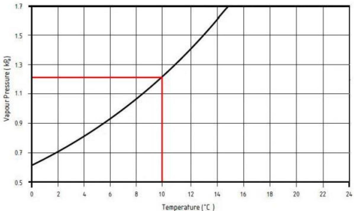
Figure 18 Graph illustrating the saturation vapour pressure (curved line) as a function of temperature and vapour pressure: in this example, the saturation vapour pressure is approx. 1.2 kPa at a temperature of 10 °C. (compare to Figure 19). (BSI, 2011, p. 21, fig. C.1 / Image © The British Standards Institution)
