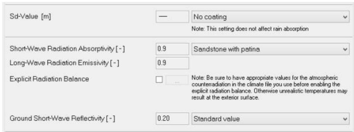
Figure 108 Screen shot of WUFI Pro showing the radiation values used in the case study simulations
