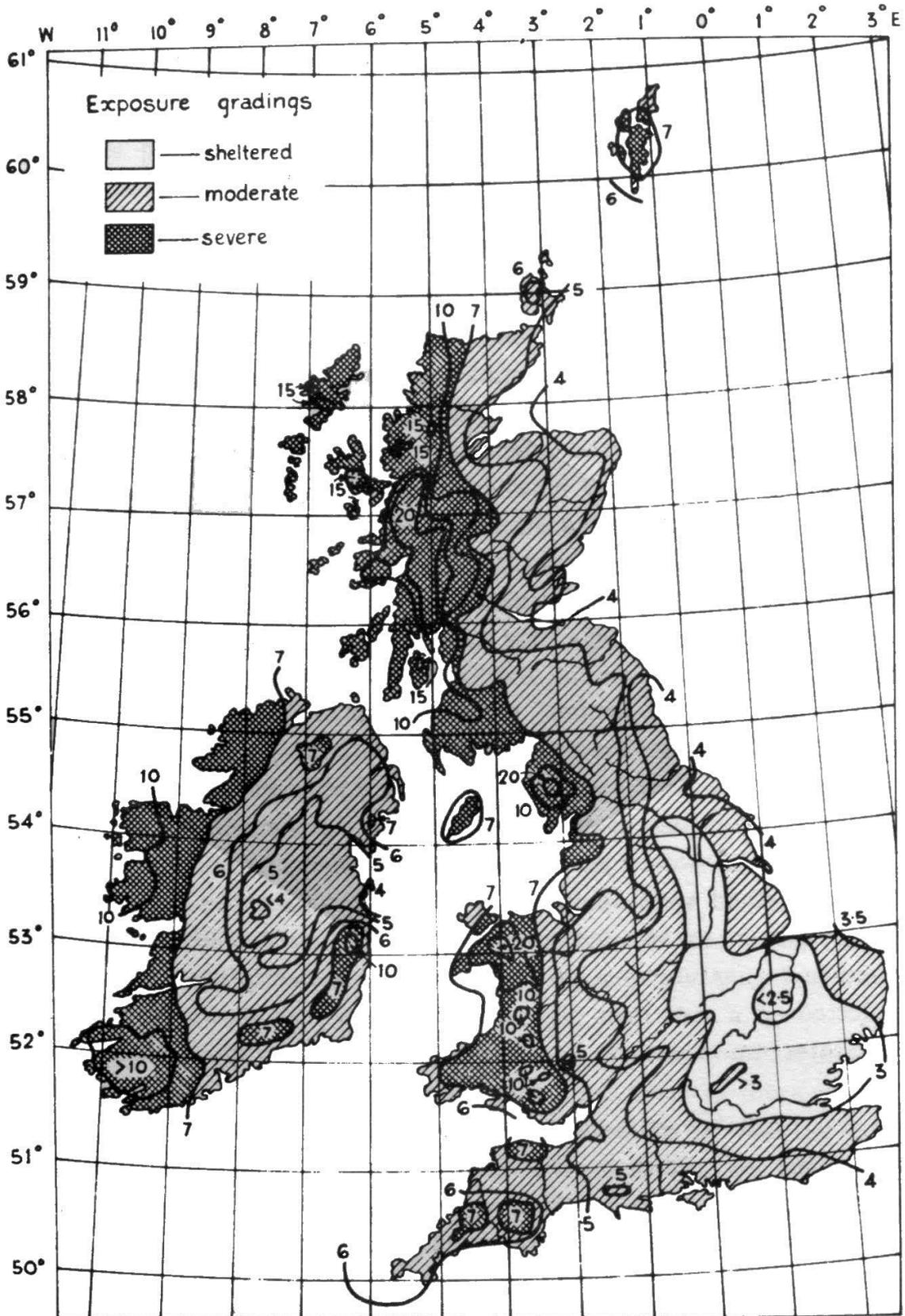
Figure 38 “Driving-rain index map of Great Britain, based on annual mean wind-speed and rainfall ( $m^2 \text{ sec}^{-1}$ )” (Lacy, 1966, p. 22, fig. 19 / Image © Building Research Establishment)
