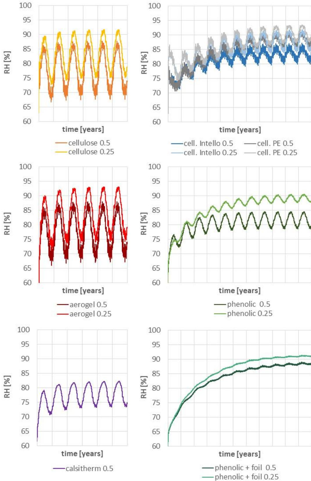
Figure 88 Relative humidity levels for the different retrofit options at the condensation critical location, namely the insulation-masonry interface, generated with WUFI using *Stone A* (The numbers behind the materials refer to the target U-values of 0.25 or 0.5 W/(m²·K).)
