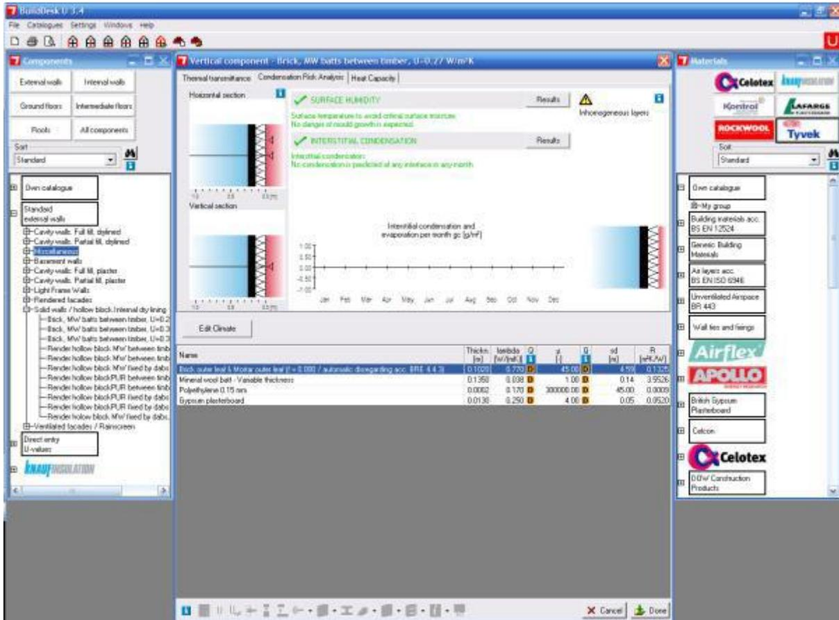
Figure 47 Screenshot of BuildDesk U 3.4: green checkmarks indicate that, according to a Glaser method assessment, no condensation is predicted.
