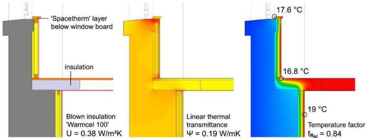
Figure 94 Cross section of a wall with a window breast, which, in comparison to Figure 93, has received additional insulation at the cill-window and floor-wall junctions: in this advanced retrofit scenario, thermal bridging has reduced significantly, surface temperatures have increased, and the temperature factor is now above the 0.75 threshold.
