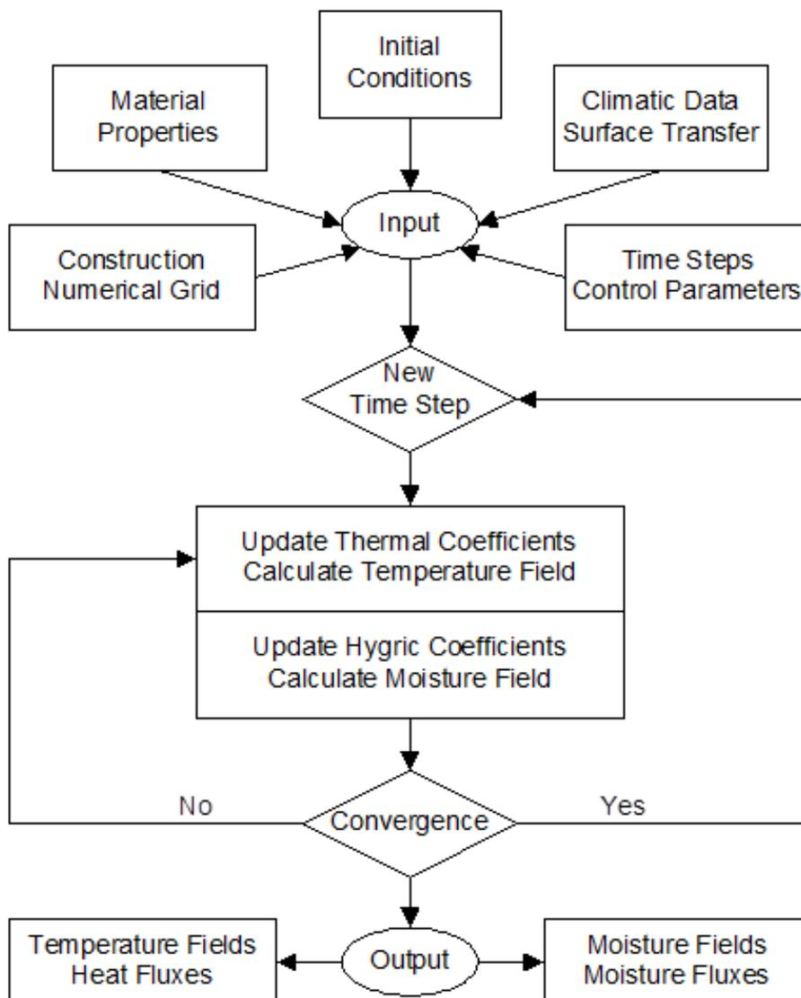
Figure 49 Flowchart illustrating the iterative process behind the numerical simulation method
