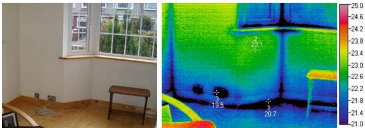
Figure 33 Photograph of an external wall with a room corner, floor junction and a bay window (left) and the corresponding thermal image (right): the thermal image shows the localised areas of lower surface temperature in blue colours. These thermally bridged areas include the outwards facing corner in the window breast, floor-wall and wall-window junctions and area where electrical sockets have been installed into the wall.
