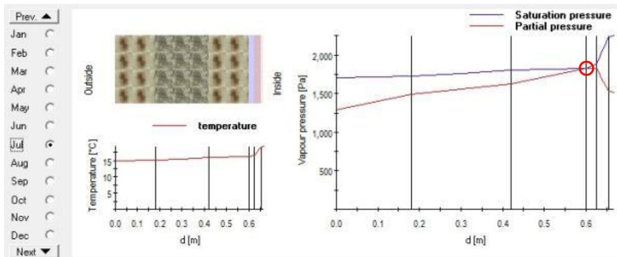
Figure 85 A partial screen shot from BuildDesk U showing the outputs of the July calculations of scenario 3.1.1 graphically, with the point of condensation circled
