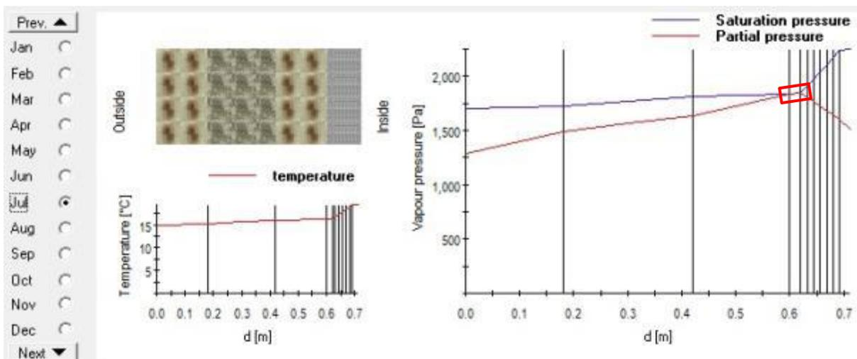
Figure 87 A partial screen shot from BuildDesk U showing the outputs of the July calculations of scenario 4.1.1 graphically, with the line of condensation marked
