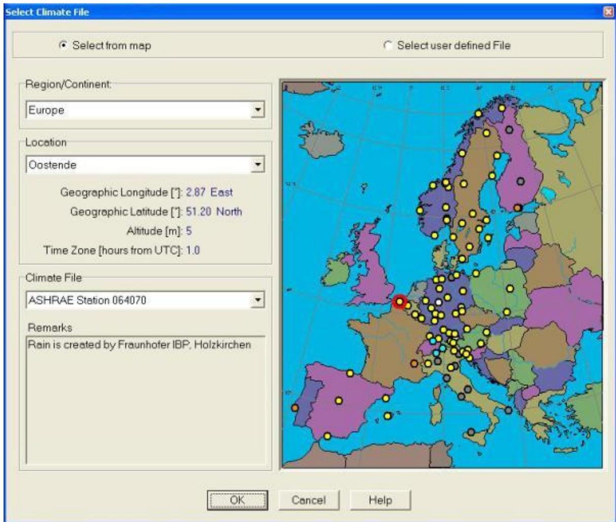
Figure 58 WUFI Pro screenshot showing the meteorological stations of Europe available within the software, with the city of Ostend (Oostende), Belgium, circled in red.
