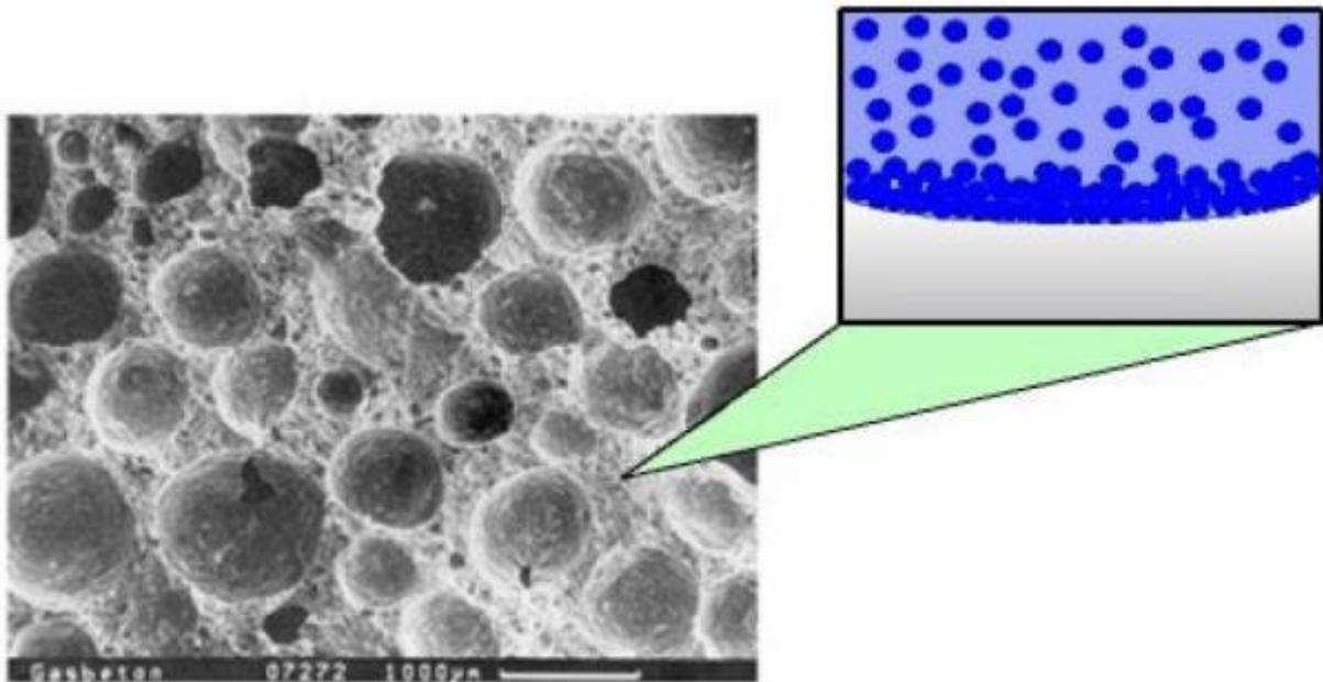
Figure 22 Microscopic photo of a pore structure and graphic illustration showing how the liquid water can adhere / be adsorbed to the surfaces of pores. (Fraunhofer IBP / Image © Fraunhofer-Gesellschaft)
