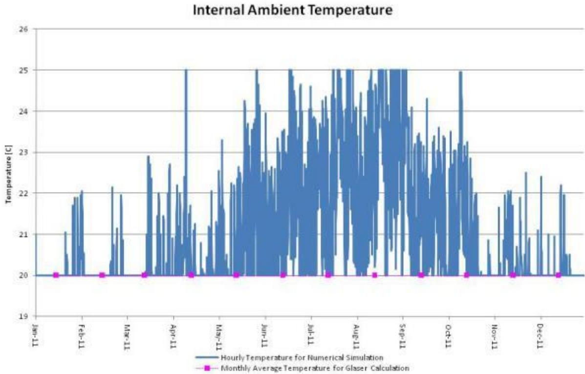
Figure 67 Indoor air temperature data used for Glaser method and numerical simulations assessments
