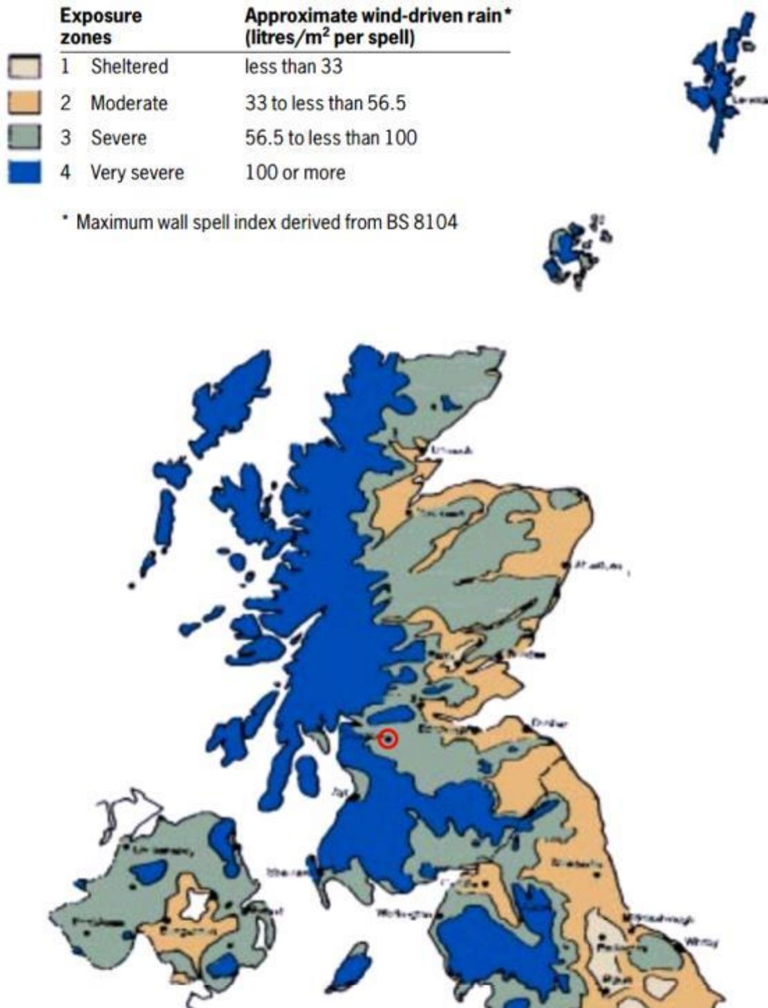
Figure 60 Map of the north of the UK with four exposure zones for wind-driven rain: Glasgow is marked with a red circle. (Image © Building Research Establishment)
