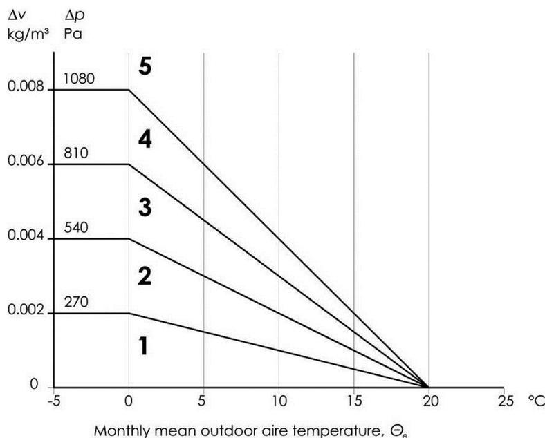
Figure 65 Correlation between indoor vapour load and outdoor air temperature for internal humidity classes, as defined in *BS EN 13788:2002* (Image © Building Standards Institute)
