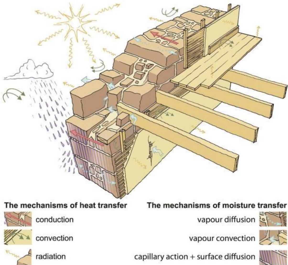
Figure 1 Mechanisms of heat transfer and moisture transport, as they occur in solid stone walls, finished internally with plaster on timber laths: the core of such masonry is made of smaller stones with a large quantity of mortar.
