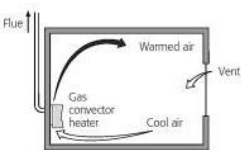
Figure 4 Convection current in a room
