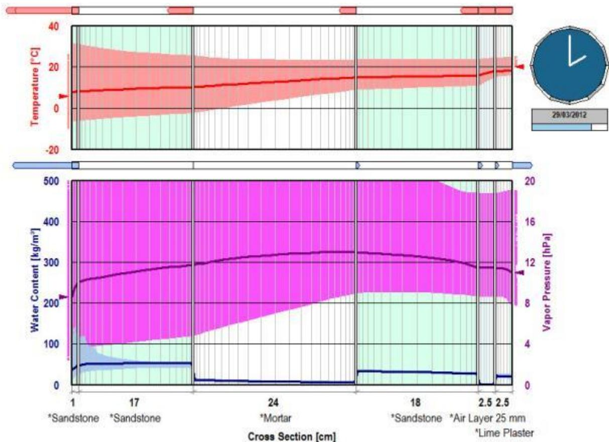
Figure 80 WUFI screenshot showing temperature, water content and vapour pressure profiles of the base wall, taken as a snapshot at a single one-hour time-step in April.
