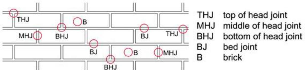
Figure 101 Positions have been marked on a drawing where tubes are to be installed.
