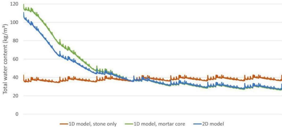
Figure 83 Total water content of the three wall models, generated with WUFI for a seven year simulation period
